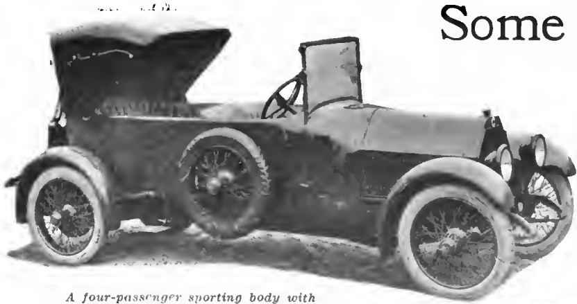
A four-passenger sporting body with Victoria top mounted on Lancia chassis. Note oval fenders, absence of running board and mounting of spare wheel
